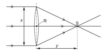
Which labelled point is the principal focus of the lens, and which labelled distance is the focal length of the lens?
